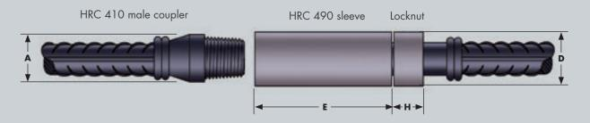
HRC 410 male coupler, HRC 490 sleeve and locknut assembled
