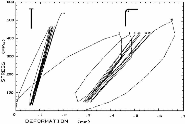
The diagram compares the stress-strain behaviour of anchorage by a HRC T-head and anchorage by bend under repeated loading and unloading between 6% and 90%  $R_{eH}$ . The T-head anchors the rebar much stiffer than a bend.
