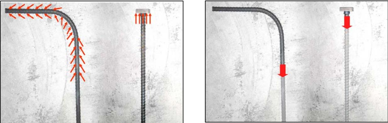
HRC 100 and 200 Series T-heads are designed to develop the tensile strength of the rebar without crushing normal strength concrete beneath the head. That makes the full capacity of the rebar available from its end. The anchorage is not dependent on bond between reinforcing steel and surrounding concrete or a crossing bar. Anchorage of the full tensile capacity of the rebar prevents premature pullout failure.
