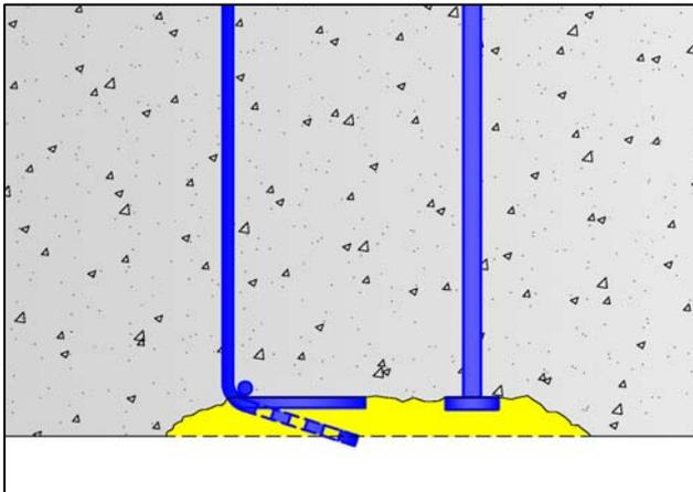
When using T-headed bars there is no danger of spalling of the concrete cover by straightening bends. In cases of lost cover the T-head can still develop the full tensile strength of the rebar. If bond is degraded in addition to spalling of the concrete cover (ex: plastic cyclic loading), the advantages of HRC T-heads can make a fundamental difference to the overall structural integrity.
