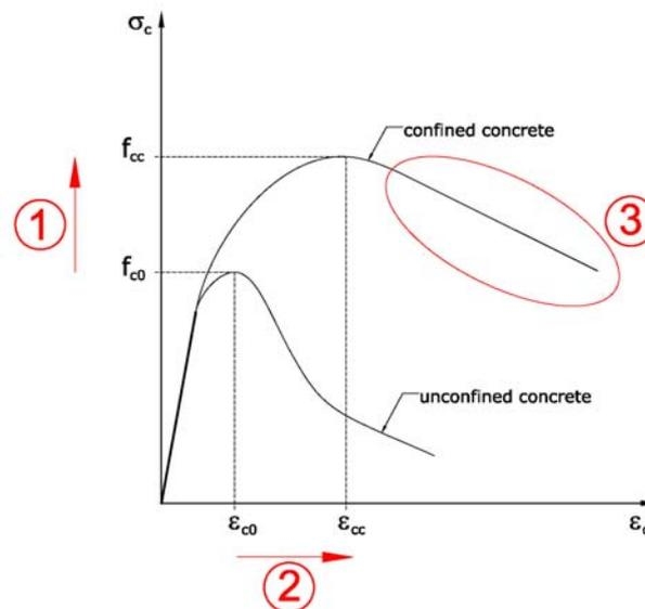
Stress-strain curve for confined and unconfined concrete
